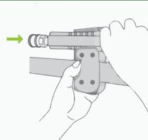
**Step 4:** Connect sprayer hose (not included in the box) to the threaded male end of the Inline Spray Gun.
