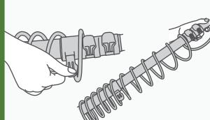
**Step 5:** Extend the Telescoping Pole to desired length by opening each clamp and pulling the pole outwards. Repeat for each of the 3 clamps. Close the clamp after extending the pole to lock into the extended position
